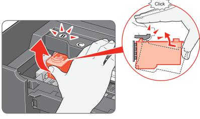
5 Repeat the procedure for the Color FINE Cartridge, inserting it into the right slot ©.
