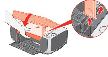
Once you have installed the FINE Cartridges, the LED will flash green. Wait until the LED stops flashing and displays 1. It takes about one to two minutes
