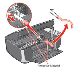
Before turning on the machine, remove all of the shipping tapes.
