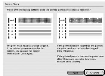
To proceed to cleaning of the Print Head, go to step 4-(3) of the Windows or Macintosh Print Head Cleaning procedure, depending on your platform. See “Print Head Cleaning” on page 33.
