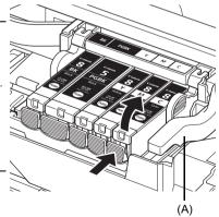
(A) Do NOT touch the Print Head Lock Lever; remove only the ink tank.
