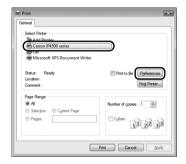
Specify the required settings and click OK. You can change the paper source to be used with the printer driver. For details, refer to "Changing the Paper Source" in the *User's Guide* on-screen manual.
