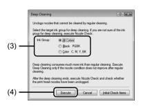
(5) Confirm the displayed message and click OK. Print Head Deep Cleaning starts when the POWER lamp starts flashing green. Do not perform any other operations until Print Head Deep Cleaning finishes. This takes about 90 seconds.
