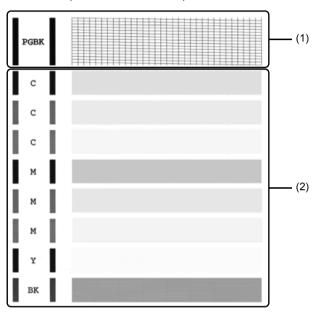
(1) If lines of this pattern are missing, the Black print head nozzle needs cleaning. Example: When lines are missing
