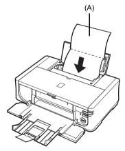
(A) Load the paper after unfolding it.
