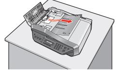
2 Lift the Scanning Unit (Printer Cover) with both hands, and pull the Scanning Unit Support down into place.
