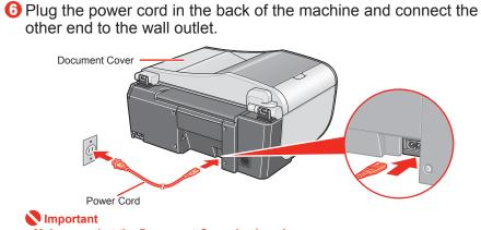
Make sure that the Document Cover is closed • Do NOT connect the USB cable at this stage.
