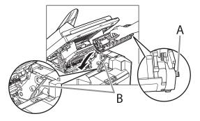
**9.** Push the toner cartridge to make sure it is properly set in the machine.
