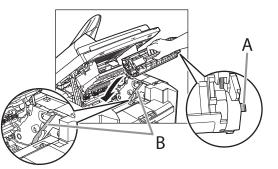
**11.** Push down the toner cartridge to make sure it is properly set in the machine.
