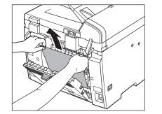
If the jammed paper is badly folded, similar to the folds of an accordion, ease the jammed paper loose and then pull it out from the machine.
