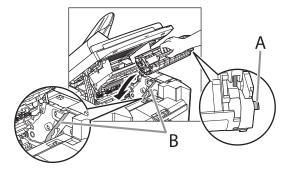
**11.** Push the toner cartridge to make sure it is properly set in the machine.
