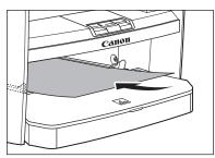
Press [◄-] or [+►] to select <FIX. UNIT CLEANING>, then press [OK].
