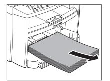
**15.** Remove the paper cassette by lifting up the front-end of the paper cassette and pulling it forward.
