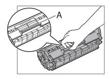
9. Insert the toner cartridge so that the protrusion on the right side of the toner cartridge (A) fits into the guide (B) located on the right side of the machine and slide it down parallel to the guide.
