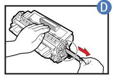
Grasp the cartridge with one hand, firmly and slowly pull out the sealing tape tab with the other hand.
