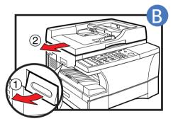
Lift the platen unit lever (1) and slide the platen unit to the left (2).
