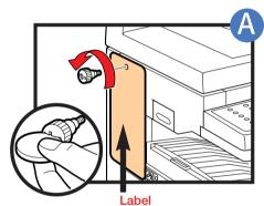
Remove the shipping attachment on the left side using a coin.
