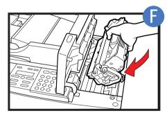
Position the arrow mark on the cartridge towards the inside of the machine, and gently slide the cartridge into the machine as far as it will go.
