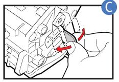
Place the cartridge on a flat and stable surface, grip the sealing tape tab and snap in the direction shown.
