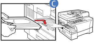
Hook the tab on the output tray onto the opening on the left side of the machine.
