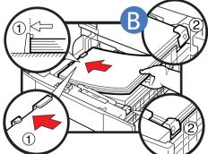
Load the paper stack beneath the cassette's length guide (1) and width guide's claws (2).
