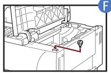
Insert the removed shipping attachment from STEP A into the holder. Keeping the cartridge
