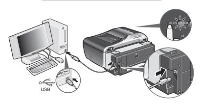
When you turn on the machine, the COPY button flashes green, then remain it. The software will begin identifying the printer port being used.
