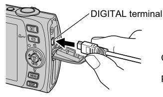
Camera: Connect the cable to the DIGITAL terminal. Printer: Refer to the printer's user guide.
