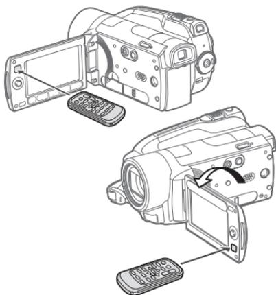
**Point the wireless controller at the camcorder's remote sensor when you press the buttons.**
