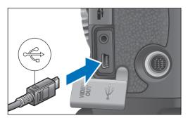
Connect with the < → > mark on the plug facing the front of the camera.
