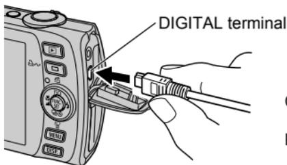
Camera: Connect the cable to the DIGITAL terminal.
