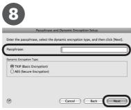
Enter your Passphrase (network password) and click Next. For the encryption method, the default setting (TKIP: Basic Encryption) should be used.
