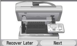
**1** Lift the scanning platform (A) until it is locked.
