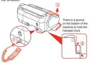
4 Connect the telephone line and any necessary external device.
