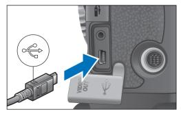
Connect the plug with the < → > mark facing the front of the camera.
