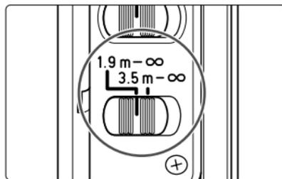
You can set the focusing distance range to 1.9 m/6.2 ft. to infinity or 3.5 m/11.5 ft. to infinity. By setting the suitable focusing distance range, the actual autofocus time can be shorter.
