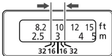
The depth of field is the distance in front of and behind the plane of focus on the subject that appears sharp. The depth of field is indicated by the area between the depth-of-field scale lines below the distance scale.
