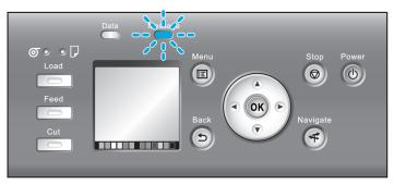
If the Data Lamp is flashing, the printer is receiving a print job. Turn off the printer only after printing is finished.
