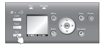
5. Press ▲ or ▼ to select Yes. As you hold the trailing edge of the printed document, press the OK button. The roll is now cut.
