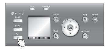
**4.** Press ▲ or ▼ to select **Yes**, and then press the **OK** button. After the roll paper is cut, it is rewound automatically.
