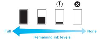
If the Display Screen indicates to replace the Ink Tank, replace the Ink Tank. If a message is displayed indicating to check the remaining ink levels, or after tasks that consume a lot of ink such as large-format printing or head cleaning, check the remaining levels and replace Ink Tank as needed. (See "Replacing Ink Tanks.") —P.984
