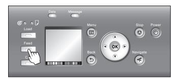
Roll paper is fed to the specified cut position and then automatically stopped.
