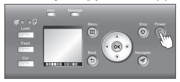
2. The **Power Lamp** is lit when the printer finishes starting up, and the printer is now in **Standby**.
