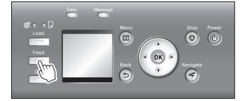
Roll paper is fed to the specified cut position and then automatically stopped.
