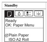
The printer is ready to receive jobs sent from the computer. Jobs sent from the computer are printed immediately.
