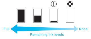
If the Display Screen indicates to replace the Ink Tank, replace the Ink Tank. If a message is displayed indicating to check the remaining ink levels, or after tasks that consume a lot of ink such as large-format printing or head cleaning, check the remaining levels and replace Ink Tank as needed. (See "Replacing Ink Tanks.") —P.997
