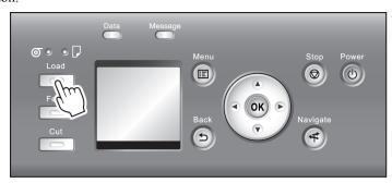
**2.** Press ▲ or ▼ to select **Load Cut Sheet**, and then press the **OK** button.
