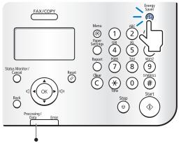
When the Processing/Data indicator is lit or blinking, the machine will not enter the Sleep mode, because an operation is in progress or an error has occurred.
