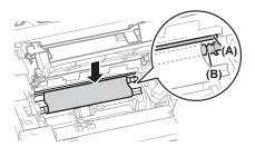
5 When the leading edge emerges, hold both sides of the jammed paper and carefully pull it out.
