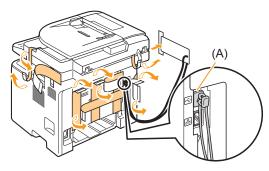
\* Do not remove the cap (A) on the USB port at this stage. Uncap when installing for USB connection.
