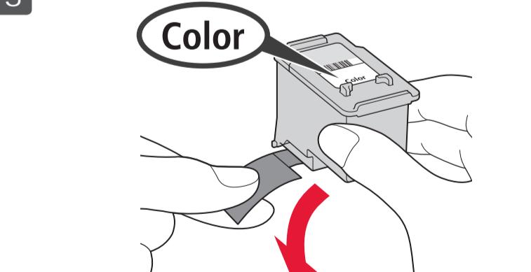
3 Unpack the FINE Cartridge, then remove the protective tape.
