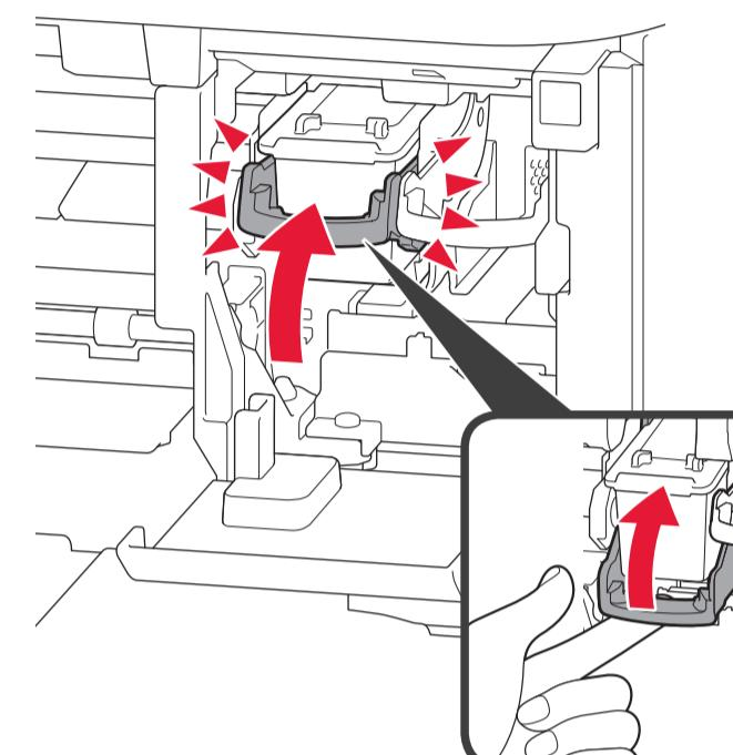
5 Lift the Ink Cartridge Lock Lever.
