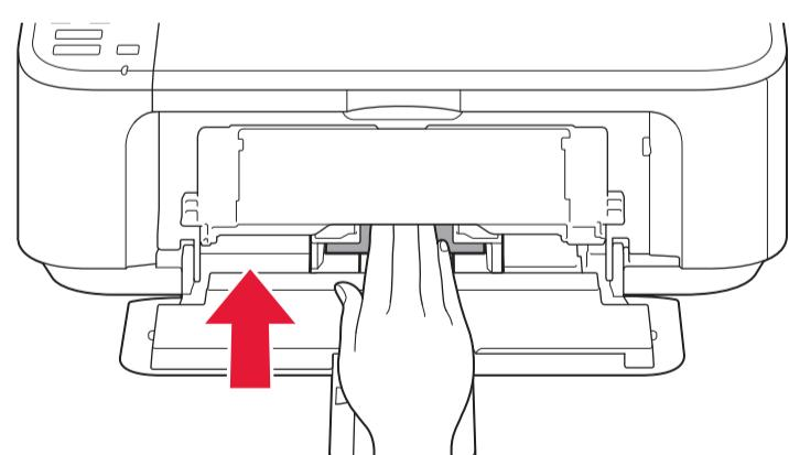
Insert paper **with the printable side down until it stops**. When using photo paper, machine settings for media type and size should be adjusted. For details, refer to the **On-screen Manual** which will be installed later.
