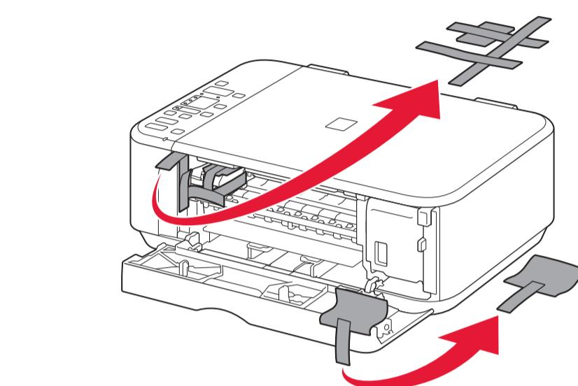
3 Remove the orange tape and protective material.
