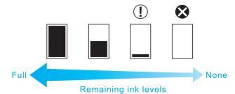
If the Display Screen indicates to replace the Ink Tank, replace the Ink Tank. If a message is displayed indicating to check the remaining ink levels, or after tasks that consume a lot of ink such as large-format printing or head cleaning, check the remaining levels and replace Ink Tank as needed. (See "Replacing Ink Tanks.")  $\rightarrow$  P.620
