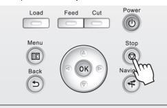
When you press the Stop button during printing, printer operation varies depending on the current status.
