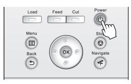
2 The **Power Lamp** is lit when the printer finishes starting up, and the printer is now in **Standby**.
