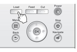
Press ▲ or ▼ to select Load Cut Sheet, and then press the OK button.
