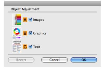
To display the Object Adjustment dialog box, click Object Adjustment on the Color Adjustment panel.
