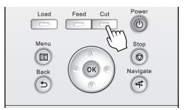
Press ▲ or ▼ to select **Yes**, and then press the **OK** button. After the roll paper is cut, it is rewound automatically.
