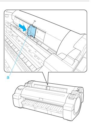
3 Load a single sheet printing-side up in the Paper Feed Slot, with the right edge aligned with the Paper Alignment Guide (a) to the right of the Roll Cover.
