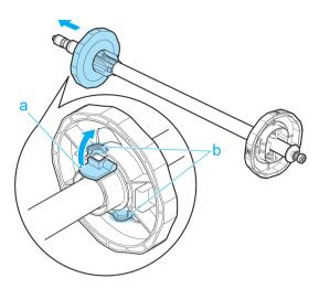
Insert the respective attachments for the roll paper core on the Roll Holder and Holder Stopper.
