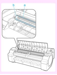
• When cleaning between the Platen and Ejection Guide, use a damp cloth that you have wrung out completely to wipe over the Output Tray and along grooves.
