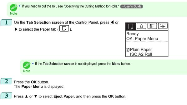
4 Press ▲ or ▼ to select "**Yes**", and then press the **OK** button. The roll is now rewound and ejected.
