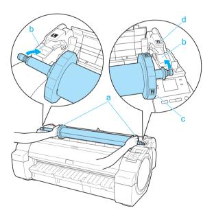
5 Holding the Roll Holder flange (a), guide the holder along the Roll Loading Slots (b) on both ends, keeping the holder level as you load it in the Roll Holder Slot.
