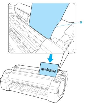
4 Move the Width Guide (a) carefully to match the size of paper loaded.
