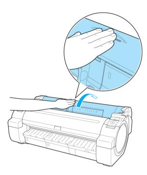
**4** Fold an A4 sheet lengthwise four times and insert it through the gap of the Paper Feed Slot. Push the scrap out toward the Platen.
