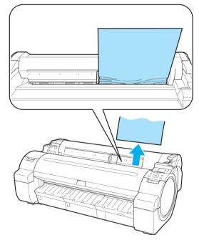
• If the paper is jammed by the Ejection Guide Remove the jammed paper from the Output Tray.
