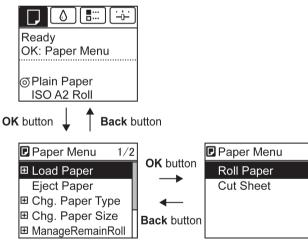
Press Back to access a higher menu in the menu list, and press OK to access a lower one. If not all menu items are displayed, hold down ▲ or ▼ to scroll through higher and lower menu items. Items you select are highlighted.
