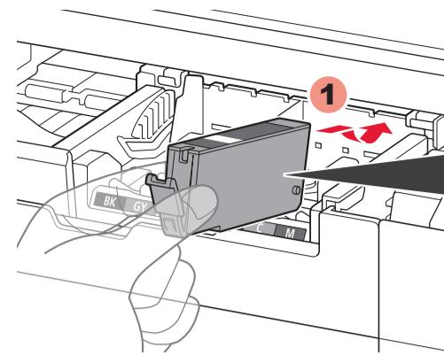
4 Insert and push down the ink tank into the matching color slot.
