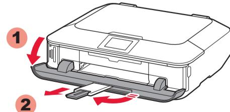
6 Open the Paper Output Tray. Pull out the Paper Output Support.
