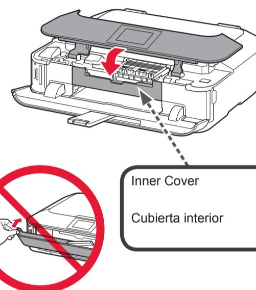
6 Check that the Inner Cover is closed, then close the Operation Panel.
