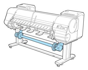
Remove tape and packaging material attached to the printer. Also open the Top Cover and remove stoppers and spacers inside the printer.
