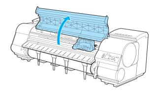
If the Cutter Unit or Carriage Cover is dirty, use a damp cloth that you have wrung out completely to wipe it clean.
