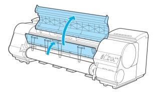
Using both hands, rotate the Roll Holder in the direction of the arrow to rewind the roll.
