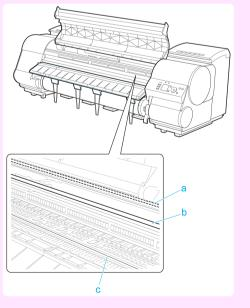
• Never touch the metal contacts of the Carriage. This may damage the printer.
