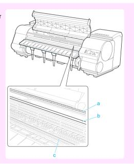
Push the Cutter Unit Detachment Lever to the left to unlock it.
