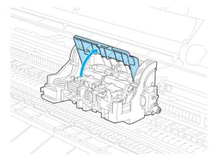
Pull the Printhead Fixer Lever forward all the way to open it completely.
