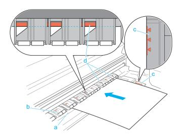
When inserted, sheets are automatically held by suction against the Platen.
