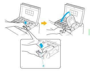
Hold the lnk Tank by the handle (a) and remove it.
