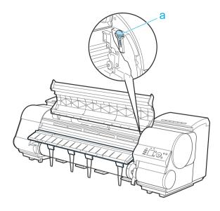
4 Using the back of the Cleaning Brush, move the first Switch to the side opposite ●.
