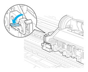
Holding the Cutter Unit by the Lock Lever (a) and grip (b), remove it from the Carriage.
