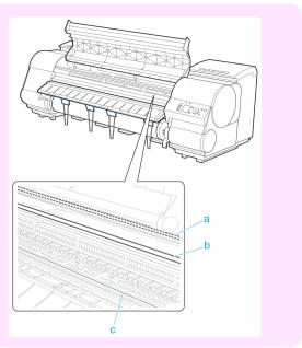
Holding the new Shaft Cleaner by the grips (a), attach it to the Carriage.
