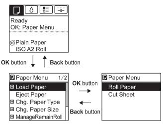
Press Back to access a higher menu in the menu list, and press OK to access a lower one. If not all menu items are displayed, hold down ▲ or ▼ to scroll through higher and lower menu items. Items you select are highlighted.
