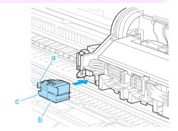
6 Lift the Cutter Unit Detachment Lever to lock it.
