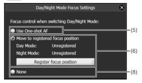
Focusing positions will vary under different light sources, such as fluorescent or infrared, since the wavelengths of these light sources vary. One of the following methods can be used to adjust the focusing position to allow for these differences when switching Day/Night Mode.
