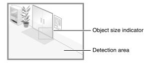
Any moving objects detected are shown with contour lines. If [Object Size (%)] and [Duration (Sec)] are not exceeded, contour lines are white. When all detection criteria are met, contour lines take on the same color as the detection area and "detected" mode is triggered to ON.
