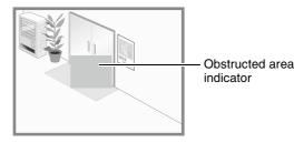
Any moving objects detected are shown with contour lines. If it is smaller than [Change Ratio (%)], contour lines are white. If the image is changed for an area larger than [Change Ratio (%)], contour lines take on the same color as the detection area, indicating that "detected" mode has been triggered to ON.
