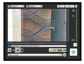
The [Start/Stop SD Card Recording] button appearance changes as shown below depending on recording status.
