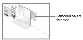
Any moving objects detected are shown with contour lines. As long as [Duration (Sec)] has not elapsed, contour lines are white. When [Duration (Sec)] has elapsed, contour lines take on the same color as the detection area, indicating that "detected" mode has been triggered to ON.
