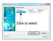
4 Enter the user name "root" and factory default setting password "camera", and then the appropriate IP address and subnet mask.
