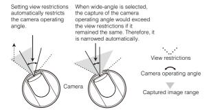
• If the view restriction will be exceeded as a result of controlling the zoom toward the wide-angle side, the camera will first pan and tilt to a position where the maximum wide-angle zoom will be within the viewing restriction area. Wide-angle zoom control will then be enabled within the view restriction area.
