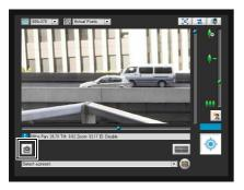
A snapshot panel will open showing a still image from the moment you clicked it. When the snapshot panel is open, click the [Get a Snapshot] button to update the image displayed in the snapshot panel.
