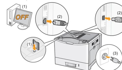
When installing or removing the optional accessories, be sure to turn the printer OFF, unplug the power plug, and then disconnect all the interface cables and power cord from the printer. Otherwise, the power cord or interface cables may be damaged, resulting in a fire or electrical shock.
