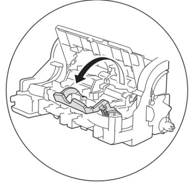
**4** Lift the printhead fixer cover to open it fully.
