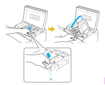
3 Hold the lnk Tank by the handle (a) and remove it.
