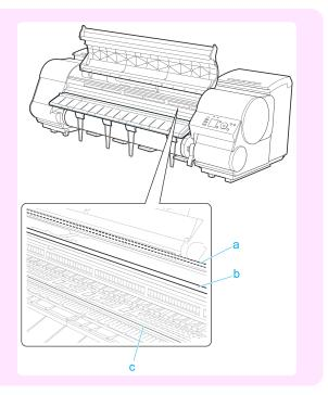
3 Push the Cutter Unit Detachment Lever to the left to unlock it.
