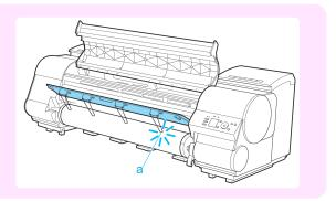
Holding the edge of the roll paper, lift the Release Lever
