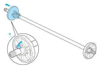
When rewinding rolls with 3-inch paper cores, insert the 3-inch Adapter on the flanges at both ends.
