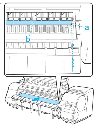
6 Lower the Release Lever and close the Top Cover.
