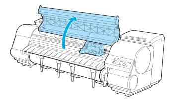
If the Cutter Unit or Carriage Cover is dirty, use a damp cloth that you have wrung out completely to wipe it clean.
