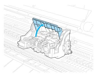
Pull the Printhead Fixer Lever forward all the way to open it completely.
