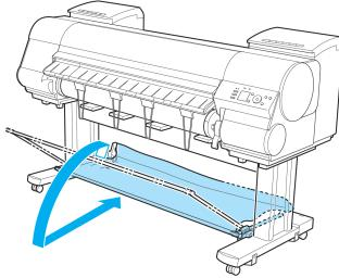
Remove the Output Stacker from the printer.
