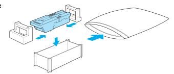
5 Confirm the Maintenance Cartridge is right-side up, put it in the box, and store it so that it stays level.
