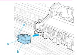
6 Lift the Cutter Unit Detachment Lever to lock it.
