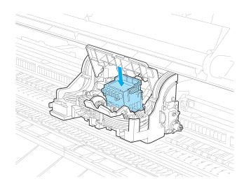
Pull the Printhead Fixer Cover down toward the front to lock the Printhead in place.
