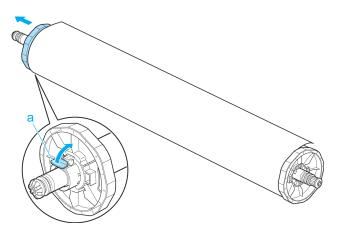
Remove the entire paper core with the rewound printed documents from the Rewind Spool.
