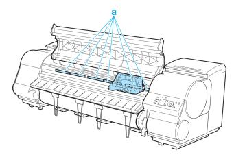
4 Pull up the Carriage Cover to open it completely.
