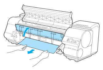
If the Carriage is on the left, move the Carriage to the right until it stops.
