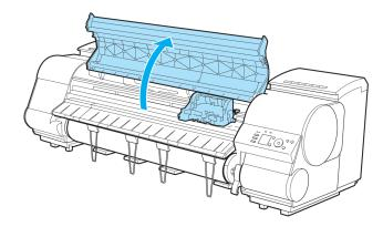
If the Carriage Cover is dirty, use a damp cloth that you have wrung out completely to wipe it clean.
