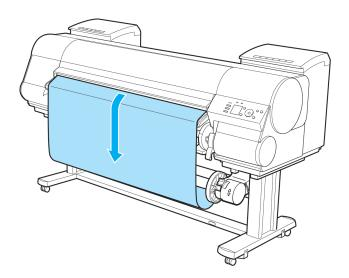
14 On the Right Media Take-up Unit, pull the Rewind Mode Switch forward to turn it on. Press the ▼ button to rewind the roll so that it is nearly taut.
