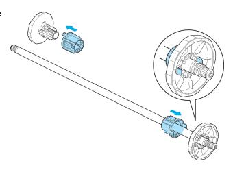
Insert the paper core, which serves as the spindle for rewinding a roll, on the Rewind Spool.
