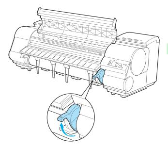
8 Hold the edge of the roll paper as you gently pull it evenly with both hands to the position of the Ejection Guide (a). Align the right side of the roll paper with the Paper Alignment Line (b), keeping this side parallel to the line, and then lower the Release Lever.
