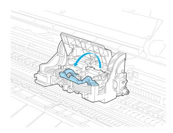
6 Pull up the Printhead Fixer Cover to open it completely.
