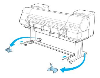
Pull out the left and right Basket Hooks from the Ejection Guide.
