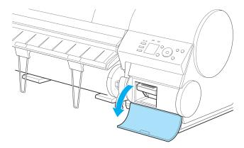
Hold the used Maintenance Cartridge by the grip (a) with one hand and put your other hand under the Maintenance Cartridge to hold it firmly on the bottom, keeping it level as you pull it out.
