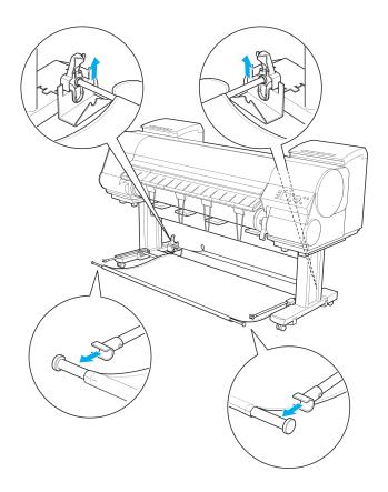
3 Stow the left and right basket arms. Next, with the Rod Holder still attached, remove the Rod Holder Adapter and put it in front of the printer.
