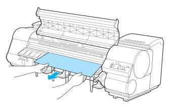
If the paper is not visible, lift the Ejection Guide, remove the Roll Holder, and clear the paper jam from below.
