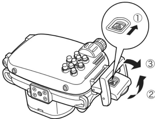
Apply a thin coat of grease to the entire seal before using the Waterproof Case in order to prevent abrasion and deterioration.
