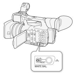
Custom white balance: You can use a white object to establish the white balance and set it to one of two custom white balance positions, ♣A or ♣B. These correspond, respectively, to positions A and B of the WHITE BAL. switch.
