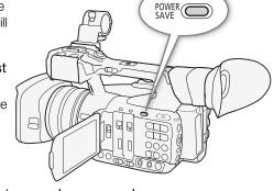
2 Press the POWER SAVE button to return the camcorder to record pause mode.
