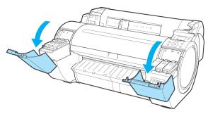
7 Load the Roll Media on the Roll Holder. (See "Attaching the Roll Holder to Rolls.") →P.12
