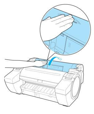
6 Using both hands, rotate the Roll Holder toward the back to rewind the roll.
