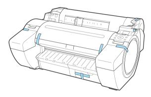
Connect the power cord to the Power Supply Connector on the right side of the printer.
