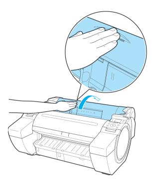
Fold an A4 sheet lengthwise four times and insert it through the gap of the Paper Feed Slot. Push the scrap out toward the Platen.
