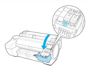
Press the tip of the lnk Tank Lock Lever of the color for replacement horizontally and pull the lnk Tank Lock Lever up to open it.
