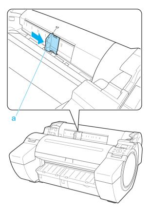
Load a single sheet printing-side up in the Paper Feed Slot, with the right edge aligned with the Paper Alignment Guide (a) to the right of the Roll Cover.
