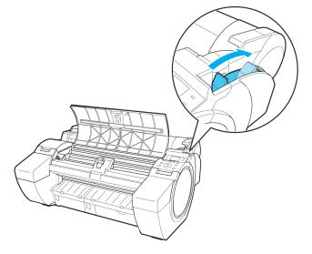
Keeping the right edge of the paper aligned with the extended line of the Paper Alignment Line (a) to the right of the ejection guide and the leading edge aligned with the groove (b) at the far end of the Platen, load the paper at the position from which to start printing.
