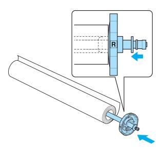
Load the roll in the printer. (See "Loading Rolls in the Printer.") >P.373
