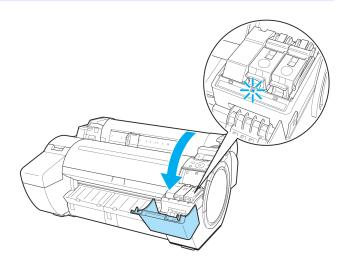
Press the tip of the Ink Tank Lock Lever of the color for replacement horizontally and pull the Ink Tank Lock Lever up to open it.
