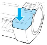
5 Open the Ink Tank Cover and check that it is attached to the printer.
