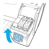
Move the Ink Tank Cover horizontally to align the position with the printer.
