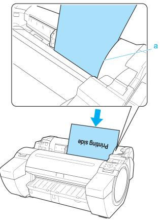
Move the Width Guide (a) carefully to match the size of paper loaded.
