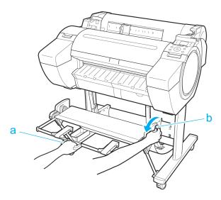
While continuing to hold the Output stacker handle (a), slowly lower the Output Stacker.
