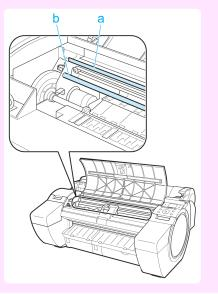
If paper from a roll is jammed by the Paper Feed Slot
