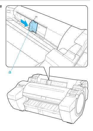
3 Load a single sheet printing-side up in the Paper Feed Slot, with the right edge aligned with the Paper Alignment Guide (a) to the right of the Roll Cover. Insert the paper until the leading edge makes contact and you hear a tone.
