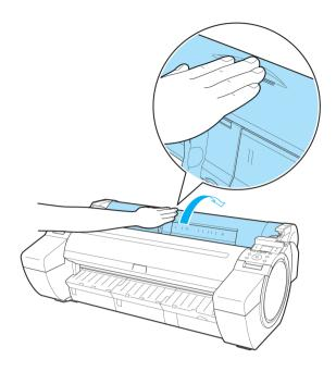
Holding the Roll Holder flange (a), rest the Roll Holder shaft on the Roll Ledge (b). At this time, position the holder so that the **R** label (c) on the [W label (c) on the Roll Holder flange is aligned with the **R** label (d) on the printer .
