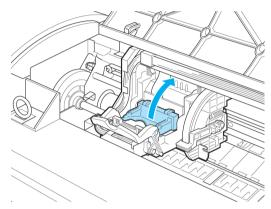
Remove the Printhead and press the **OK** button.
