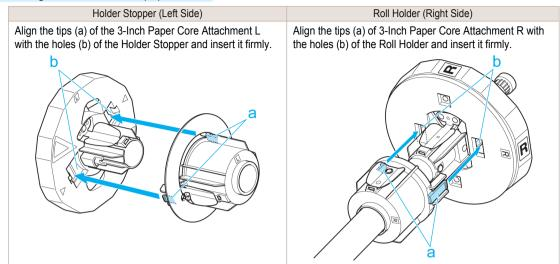
With the edge of the roll paper facing forward as shown, insert the Roll Holder from the right of the roll. Insert it firmly until the roll touches the flange (a) of the Roll Holder, leaving no gap.
