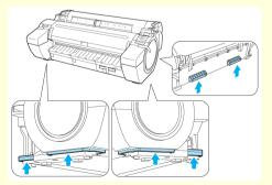
• When placing the printer on the Stand, lock all four of the casters of the Stand. Attempting to place the printer on the Stand while the casters are not locked poses a risk of injury.
