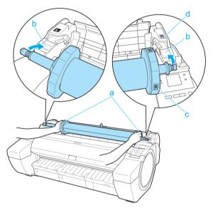
Holding the Roll Holder flange (a), guide the holder along the Roll Loading Slots (b) on both ends, keeping the holder level as you load it in the Roll Holder Slot.
