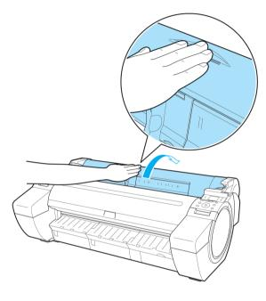
Using both hands, rotate the Roll Holder toward the back to rewind the roll.
