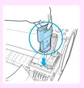
4 Push the lnk Tank Lock Lever closed until it clicks into place.
