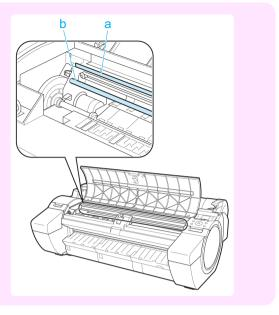
If the paper is jammed by the Paper Feed Slot Remove the jammed paper from the Paper Feed Slot.
