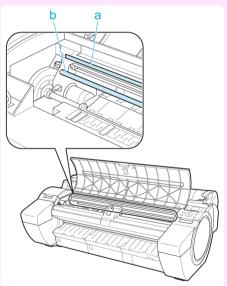
• Never touch the metal contacts of the Carriage. This may damage the printer.
