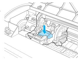
Pull the Printhead Fixer Cover down toward the front to lock the Printhead in place.
