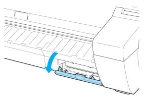
Hold the used Maintenance Cartridge by the grip (a) with one hand and put your other hand under the Maintenance Cartridge to hold it firmly on the bottom, keeping it level as you pull it out.
