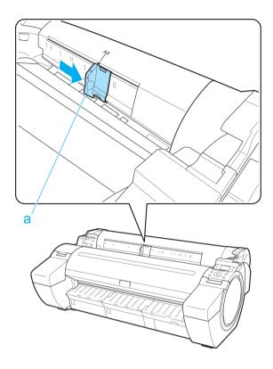
Load a single sheet printing-side up in the Paper Feed Slot, with the right edge aligned with the Paper Alignment Guide (a) to the right of the Roll Cover.
