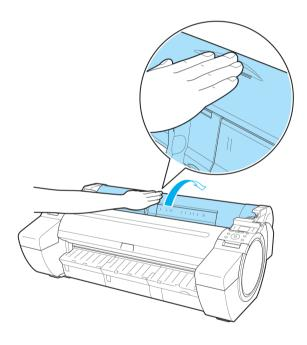
2 Cut the loaded roll paper with regular scissors or the like.
