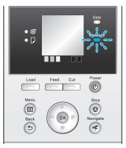
If the **Data Lamp** is flashing, the printer is receiving a print job. Turn off the printer only after printing is finished.
