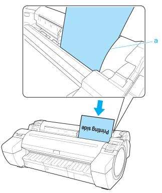
Move the Width Guide (a) carefully to match the size of paper loaded.
