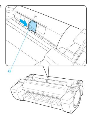
Load a single sheet printing-side up in the Paper Feed Slot, with the right edge aligned with the Paper Alignment Guide (a) to the right of the Roll Cover. Insert the paper until the leading edge makes contact and you hear a tone.
