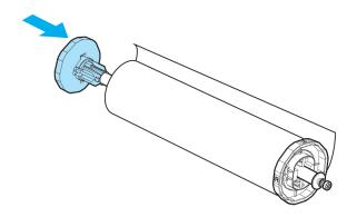
Load the Roll Media in the printer. (See "Loading Rolls in the Printer.") →P.375
