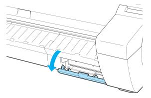
Hold the used Maintenance Cartridge by the grip (a) with one hand and put your other hand under the Maintenance Cartridge to hold it firmly on the bottom, keeping it level as you pull it out.
