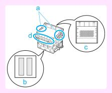
While firmly holding the Printhead you have removed, use your other hand to remove the orange Protective Part (a). Squeeze the grips (c) of Protective Part (b) and pull it down to remove it.
