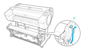
When using 24-inch or A1 (portrait) roll paper, pull out the Adjustable Stopper (a). This completes the procedure for switching to Extended position A.
