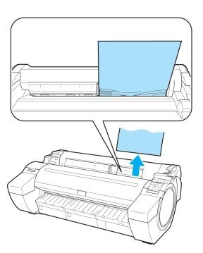
If the paper is jammed by the Ejection Guide
