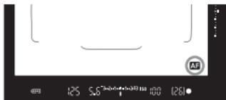
When you press the shutter button halfway and the camera is focusing with AF, the <AF> icon will appear on the lower right of the viewfinder.
