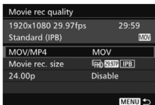
With [**4**: **Movie rec quality**] (the [**2**] tab in <[+] >), you can set the movie recording format, movie recording size (size, frame rate, compression method), and other functions.
