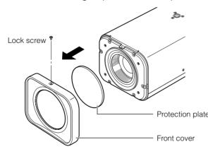
• When reattaching the protection plate, face the side with the cutout toward the lens.
