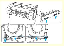
• When placing the printer on the Stand, lock all four of the casters of the Stand. Attempting to place the printer on the Stand while the casters are not locked poses a risk of injury.
