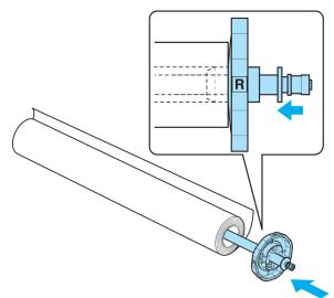
3 Load the roll in the printer. (See "Loading Rolls in the Printer.") →P.322
