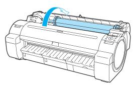
Holding the Roll Holder flange (a), remove the holder from the Roll Holder Slot.
