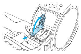
Hold the lnk Tank by the grips and remove it. Press the **OK** button.
