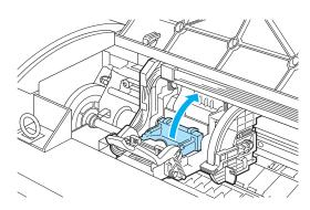
5 Remove the Printhead and press the **OK** button.
