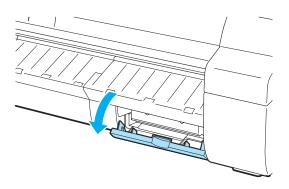
3 Hold the used Maintenance Cartridge by the grip (a) with one hand and put your other hand under the Maintenance Cartridge to hold it firmly on the bottom, keeping it level as you pull it out.
