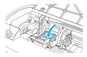
Push the Printhead Fixer Lever toward the back of the printer until it clicks.
