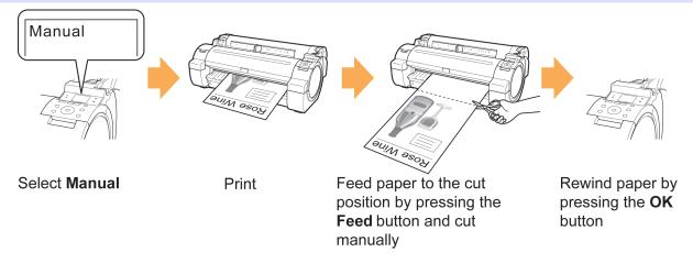
On the **Tab Selection screen** of the Control Panel, press **◄** or **▶** to select the Paper tab (□).
