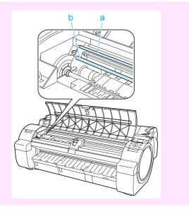
Pull the Printhead Fixer Lever forward all the way to open it completely.
