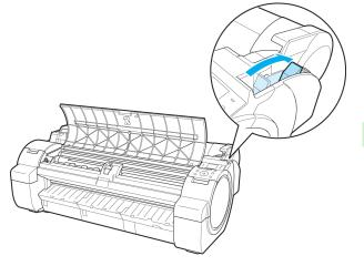
Keeping the right edge of the paper aligned with the extended line of the Paper Alignment Line (a) to the right of the ejection guide and the leading edge aligned with the groove (b) at the far end of the Platen, load the paper at the position from which to start printing.
