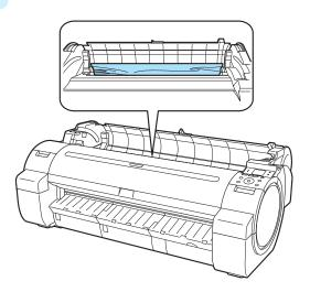
If the paper is jammed by the Ejection Guide Remove the jammed paper from the Output Tray.
