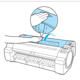
Using both hands, rotate the Roll Holder toward the back to rewind the roll.
