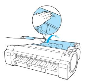
Fold an A4 sheet lengthwise four times and insert it through the gap of the Paper Feed Slot. Push the scrap out toward the Platen.
