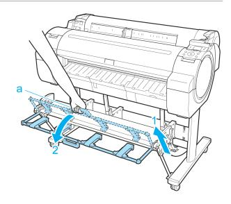
Open the Output Stacker Ejection Guides (a). This completes the procedure of switching to Extended position B.
