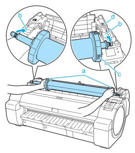
Holding the Roll Holder flange (a), guide the holder along the Roll Loading Slots (b) on both ends, keeping the holder level as you load it in the Roll Holder Slot.
