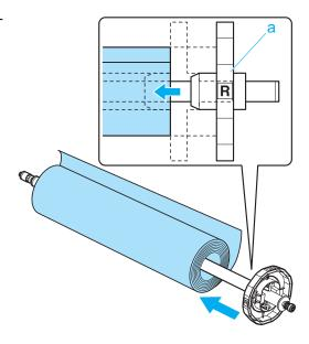
Insert the Holder Stopper from the left in the Roll Holder as shown. Holding it at the position shown (b), push it firmly in until the flange (a) of the Holder Stopper touches the roll. Lock the Holder Stopper lever (c) by pushing it down toward the shaft side.
