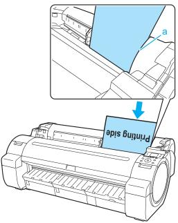
Move the Width Guide (a) carefully to match the size of paper loaded.
