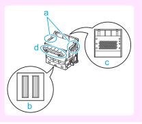
While firmly holding the Printhead you have removed, use your other hand to remove the orange Protective Part (a). Squeeze the grips (c) of Protective Part (b) and pull it down to remove it.
