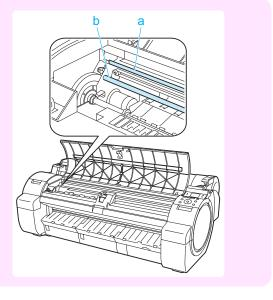
If paper from a roll is jammed by the Paper Feed Slot
