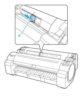
3 Load a single sheet printing-side up in the Paper Feed Slot, with the right edge aligned with the Paper Alignment Guide (a) to the right of the Roll Cover.
