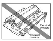
• Do not hold or touch the imaging transfer belt. The image quality may deteriorate. Do not apply shock to the drum cartridge memory or bring it near magnetic waves. It may result in damage to the machine.
