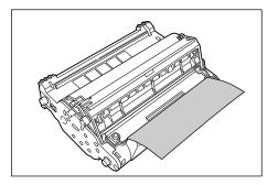
Turn the knob on the drum cartridge in the direction of the arrow.
