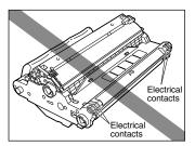
Do not hold or touch the imaging transfer belt. The image quality may deteriorate. Do not apply shock to the drum cartridge memory or bring it near magnetic waves. It may result in damage to the machine.
