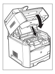
If the message is still displayed after closing the cartridge cover and lowering the scanning platform, proceed to the following procedure.
