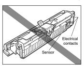
• Do not touch or hold the development roller. The image quality may deteriorate. Do not apply shock to the toner cartridge memory or bring it near magnetic waves. It may result in damage to the machine.
