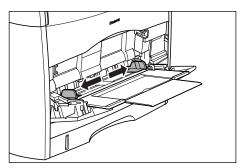
3 Gently load the stack of paper with the printing side facing up until it touches the back of the tray.
