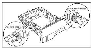
**3** Hold the lock release lever of the rear paper guide and slide the guide to the mark indicating the subject paper size.
