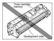
• When handling a toner cartridge, hold it properly as shown in the figure. Do not set it vertically or upside-down.
