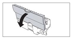
17 Tilt both the green pressure release lever on the left and right side of the fuser unit towards you to release the pressure in the fuser unit.
