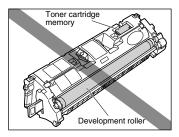
• Keep the protective cover with which the cartridge from removed. It may be required when taking out the toner cartridge for machine maintenance.
