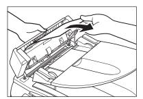
**2** Widen the document guides until they stop, and remove the paper so as not to be caught by the guides. Open the ADF and gently remove the jammed paper from the ADF.
