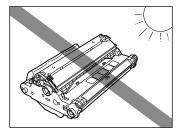
• Do not hold or touch the electrical contacts. It may result in damage to the machine.
