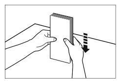
6 Gently load the stack of envelopes with the address side facing up and the flap side come the leftward. Be sure to insert the envelopes completely.
