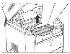
If paper is jammed in the removed drum cartridge, do not try to pull the paper out forcefully but see "Paper Jam in the Drum Cartridge," on p. 9-21.
