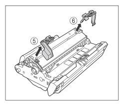
Hold the packing material 7 and remove it as shown in the figure.
