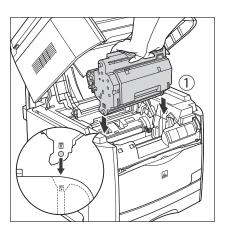
Lock the drum cartridge by pushing it down toward you ②.
