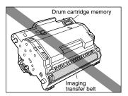
8 Place the drum cartridge in the protective bag.
