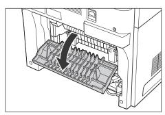
2 Tilt both the green pressure release lever on the left and right side of the fuser unit towards you to release the pressure in the fuser unit.
