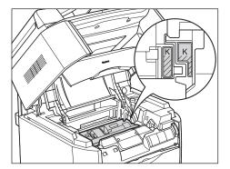
If the spent toner cartridge is not in the replacement position, close the cover, then open it again when the whirring sound stops. Repeat this process until the cartridge you want to replace is in the correct position.
