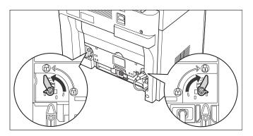
15 Hold the grip on the fuser unit and remove it.
