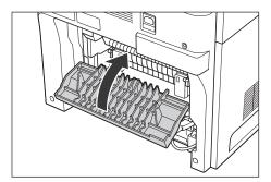
14 Turn the lock release levers located on the back of the machine in the direction of the arrow and release the lock.
