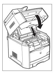
If the message is still displayed after closing the cartridge cover, pieces of torn paper may still be remaining inside. Re-check the various sections of the machine and remove all pieces of the jammed paper from inside the machine.
