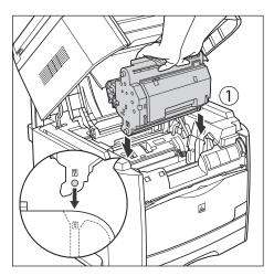
Lock the drum cartridge by pushing it down toward you 2.
