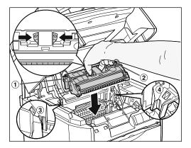
When the toner cartridge is installed properly, the label on the cartridge and on the toner cartridge holder will be aligned as shown in the figure.
