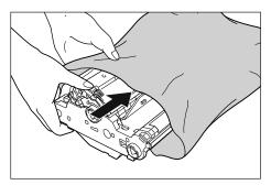
**9** Press the green lock release lever ① and remove the jammed paper 2.
