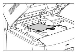
2 If paper is jammed in the multi-purpose tray, remove the jammed paper.
