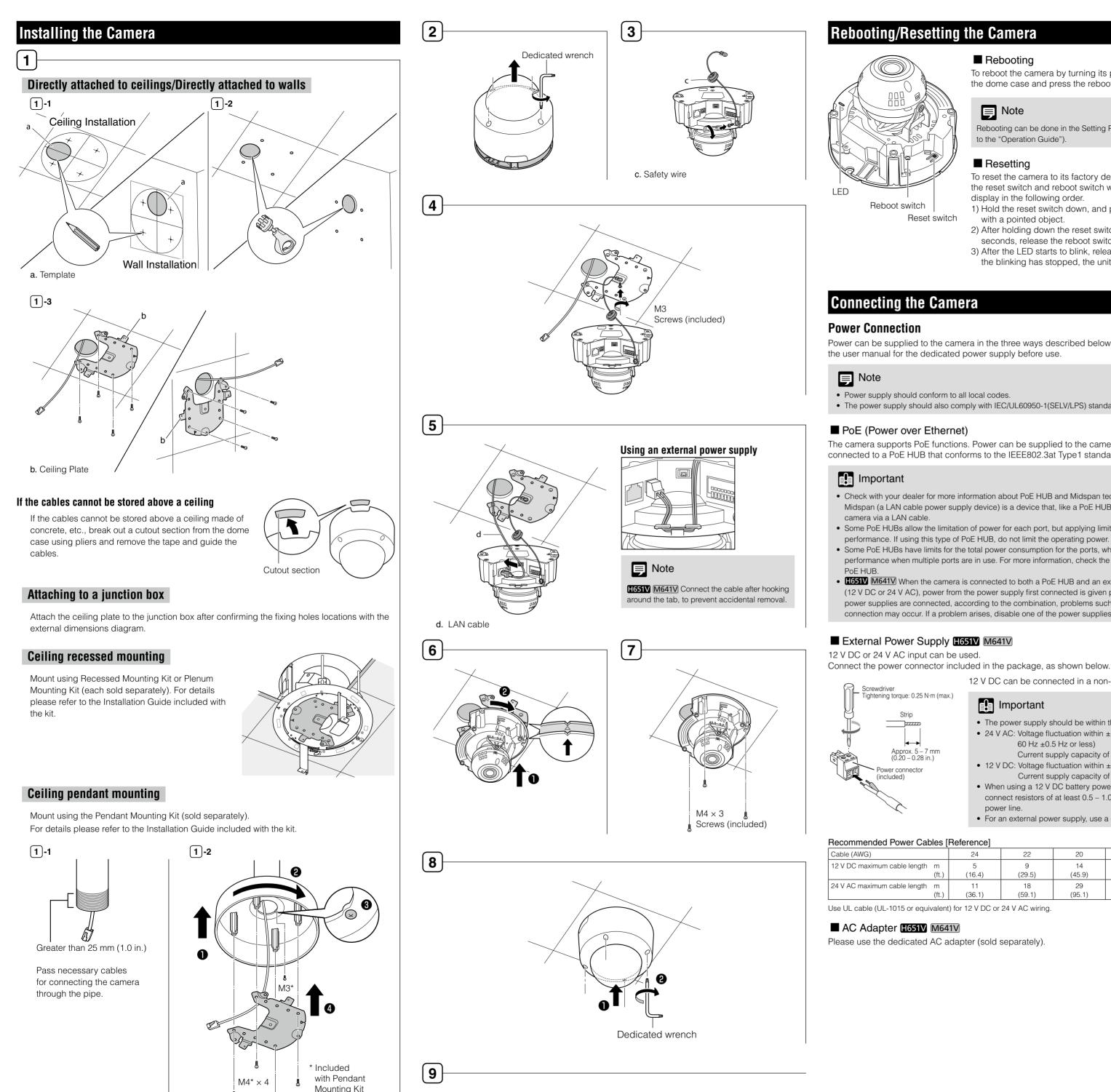
When the installation has finished, please adjust the camera angle as needed. For more information, please refer to the "Operation Guide".
