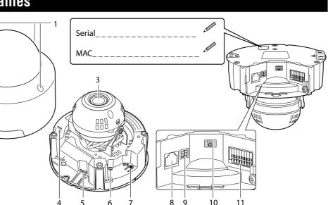
1. Dome case lock screw / 2. Dome case / 3. Lens unit / 4. LED (Blue)\* / 5. Memory card slot / 6. Reboot switch / 7. Reset switch / 8. 100Base-TX LAN connector / 9. Power connection terminal H651V M641V / 10. Audio I/O terminal H651V M641V 11. External device I/O terminals H651V M641V
