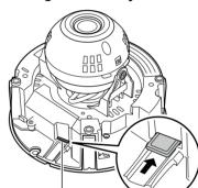
Remove the dome case and place the memory card in the memory card slot.
