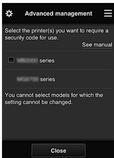
Each user can set a [Security code](#), start the app, and perform printing and other operations. This setting is linked with **Multuser mode** on the **Mng. printer** screen.
