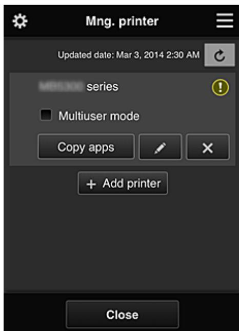
From the **Mng. printer** screen, you can [check](#) or [update](#) printer information registered to the Canon Inkjet Cloud Printing Center, [copy apps](#), [change printer names](#), [delete printers](#), and [add printers](#).
