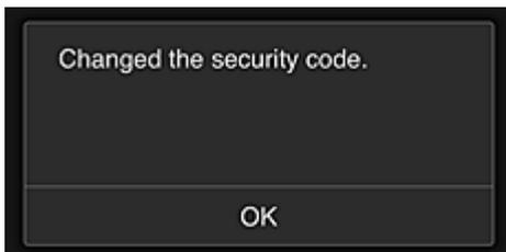
The **Security code** change process ends, and the change completion message appears. In the message screen, select **OK** to return to the main screen.
