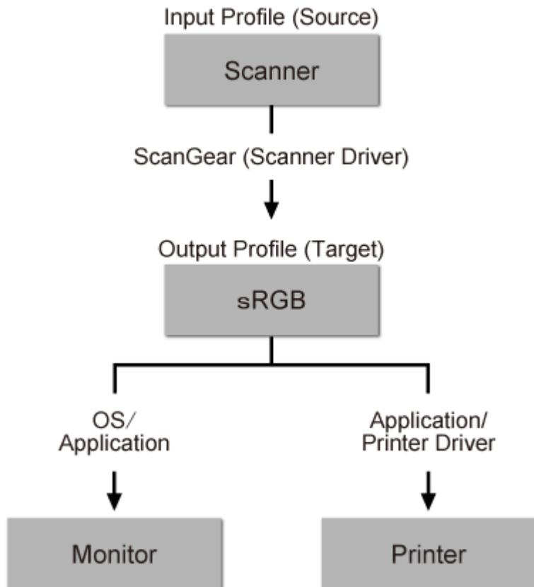
The image's color space is converted from the scanner's color space to sRGB by ScanGear.
