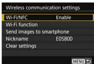
The **[Wireless communication settings]** screen displayed in step 4 on page 17 is the portal screen for setting the wireless functions.
