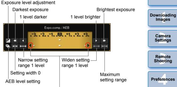
When the AEB bracketing setting exceeds the displayable range, [4], [▶] marks are displayed to show there are bracketing indicators beyond the scale.
