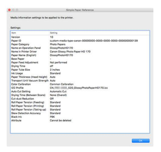
The information that will appear in the Simple Paper Reference dialog box is media information sent by the Media Configuration Tool. After updating the media information with the Media Configuration Tool, check the printer control panel to verify the media information values that were changed in the printer control panel.
