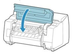
5. Tape down printer covers to secure them, in the reverse order of tape removal during installation.
