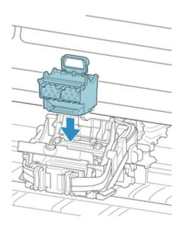
11. Lower print head locking cover to front and lock print head.
