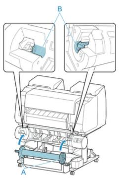
8. Change Roll Holder Lock switch on roll unit to lock direction.
