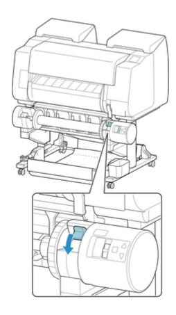
9. Change the feed flap switch on top of the roll unit so that the switch indicator (A) is aligned with ● (B) position on the take-up icon.
