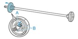
3. If taking up roll paper whose paper core has an inner diameter of 3 inches (76.2 mm), insert 3-Inch Paper Core Attachment in roll holder and holder stopper.
