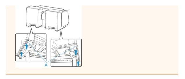
2. Remove tape and packaging material attached to the printer. Also open the top cover and remove stoppers and spacers inside the printer.
