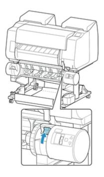
7. Hold flanges (A) so that roll holder's white gear is on left, align roll holder shaft with roll holder slot left and right guide grooves (B), and load.
