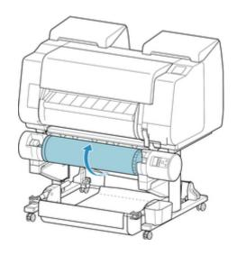
6. Change Roll Holder Lock switch on roll unit to release position.
