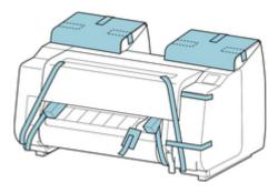
3. If using optional roll unit, refer to Setup Guide provided with roll unit and attach roll unit to Stand.
