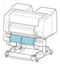
Apply adhesive tape to the rewound paper to hold it in place, if necessary.
