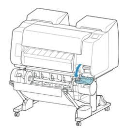
3. Hold the used maintenance cartridge by the grip (A) with one hand and put your other hand under the maintenance cartridge to hold it firmly on the bottom, keeping it level as you pull it out.
