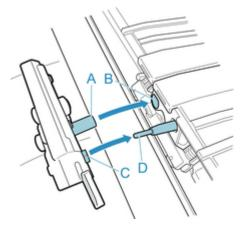
6. Install while aligning fixing part included with replacement cutter blade with center of cutter blade.
