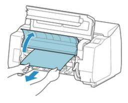
After removing the paper, inspect the interior to ensure paper fragments or other objects do not remain, and lower the output guide.
