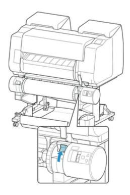
9. Hold roll holder by its flanges (A), and remove from roll unit.
