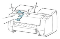
• Open top cover and output guide and clean parts that come in contact with paper (A, B).
