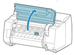
2. If cutter blade is dirty, use damp cloth that you have wrung out completely to wipe it clean.
