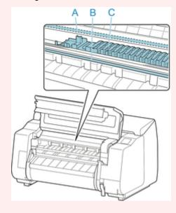
3. If ventilation duct (A) is dirty, use damp cloth that you have wrung out completely to wipe it clean.
