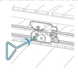
4. Remove cutter blade while holding A.
