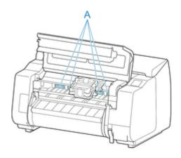
4. While pressing button (A) in center of print head lock lever, pull it forward to open it until it stops.
