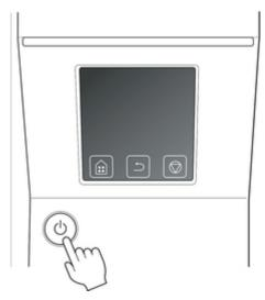
2. When startup is finished, **ON** button lights up, and printer enters standby mode.
