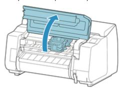
2. If the print head locking cover and print head lock lever are dirty, use a damp cloth that you have wrung out completely to wipe them clean.
