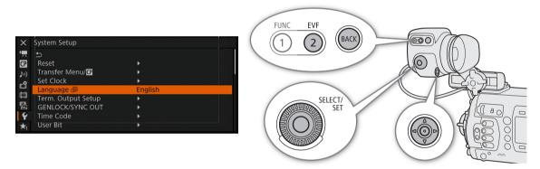
EVF button: Open the monitoring menu. On the RC-V100, press the MENU button instead.
