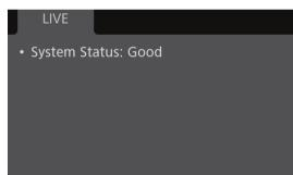
When the INFO icon M appears on the control display, open the **INFO** > [LIVE] screen to check important information regarding the status of the camera. If there are no problems with the camera, [System Status: Good] will be displayed. If an error message appears on this screen, check the list of messages ( $\fbox{224}$ ).
