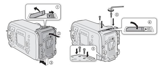
1 Slide the battery adapter release switch in the direction of the arrow.
