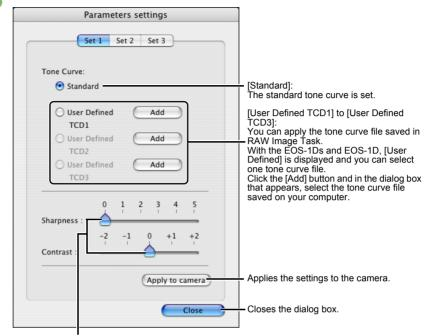
Drag the slider left or right to specify the sharpness and contrast. With the EOS-1Ds and EOS-1D, [Sharpness] and [JPEG Quality] are displayed. Select the item to be set from the list box.
