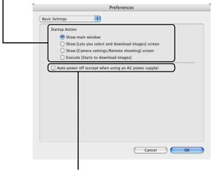
Check this checkbox to enable the Auto power off function.
