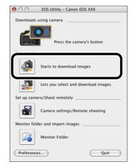
The above window shows information displayable when EOS 30D or EOS DIGITAL REBEL XTI/400D DIGITAL is connected. The displayed information varies depending on the camera model connected.
