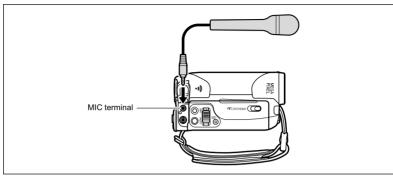
O You can connect almost any stereo microphone equipped with a Ø3.5 mm plug but the audio level will be different than with the built-in microphone.
