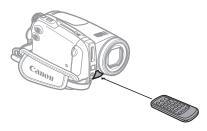
Point the controller at the camcorder's remote sensor when you press the buttons.
