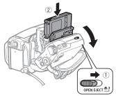
1 Slide OPEN/EJECT ★ fully in the direction of the arrow and open the cassette compartment cover.
